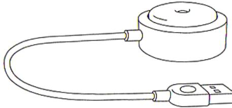
First, connect the battery to the charger, via USB cable. Remove tracker from the strap and place it on the induction stand side without inscription upward. A blinking white light indicates the middle of beginning of charge when the device is fully charged, the white LED will lit continuously.
